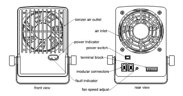
The front panel of the ElimStat Micro has two LED indicator lights. The green LED indicates the unit is powered. The red LED is a fault indicator for the high voltage power supply monitoring circuit. The high voltage power supply monitoring circuit also drives the fault alarm relay.
