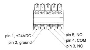
The plug type terminal block also provides relay contact output for the fault alarm. Pin 4 is Common. Pin 5 is Normally Open. Pin 3 is Normally Closed. The relay contacts are rated for a maximum of 1 A at 30 Vdc resistive with a maximum switching voltage of 220 VDC.
