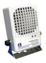
The Elimstat Micro ionizing air blower utilizes steady-state DC corona ion technology across 6 stainless steel emitters. Its small footprint allows it to be mounted inside machine enclosures and locations with restricted surface mount area.
